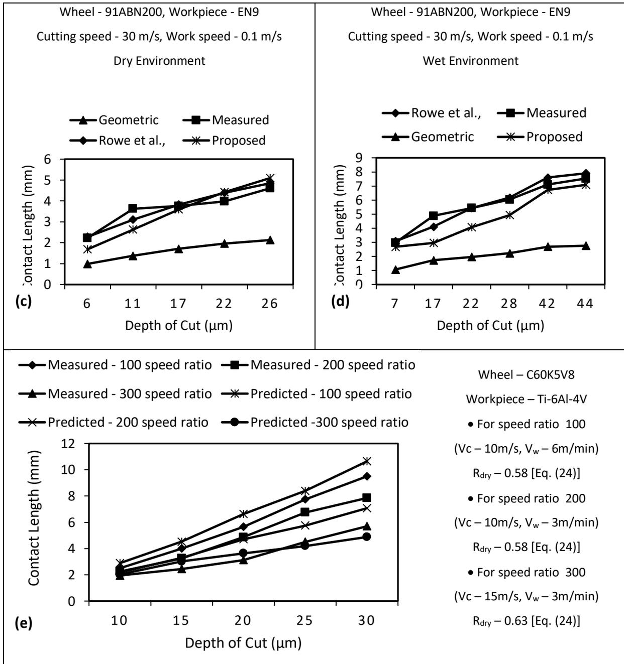
Figure.3 (a, b, c, d) Summary of experimentally measured contact length, calculated contact length using Rowe and Qi formula, geometric contact length and calculated contact length using propose formula at different kinematic conditions. (Measured and Rowe et al., data is from Rowe and Qi<sup>2, 13</sup>) (e) Evaluation of proposed model by additional experiments
