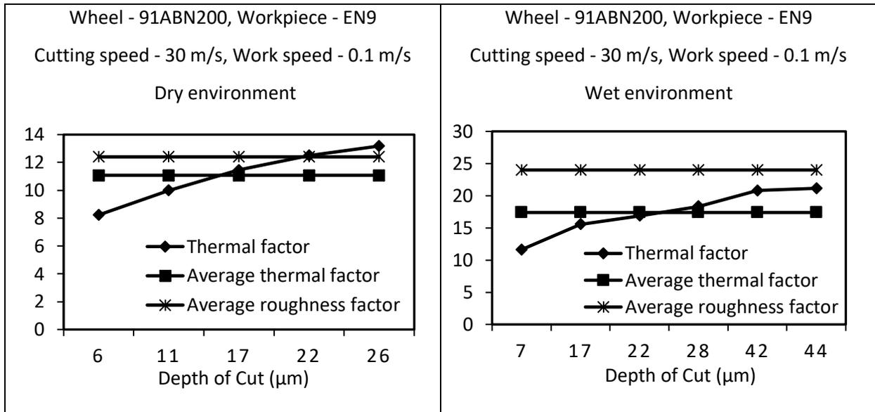
Figure. 1 Average roughness factor, thermal factor and average thermal factor values for different grinding conditions (Average roughness factor data from Rowe and Qi<sup>2, 13</sup>)
