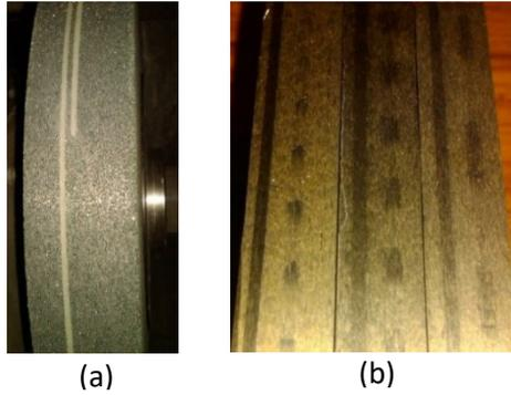
Figure 2. (a) Slots on wheel surface (b) Pattern on surface after first pass
